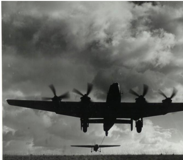
A Halifax bomber on take-off towing a Horsa Glider Photo courtesy IWM, UK.
