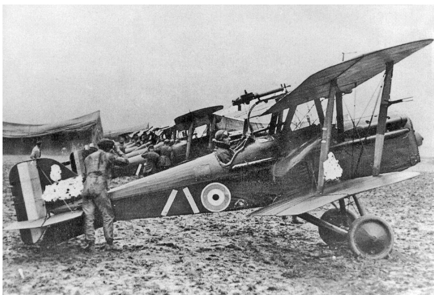
Royal Aircraft Factory S. E. 5a of Number 2 Squadron Australian Flying Corps (AFC)
