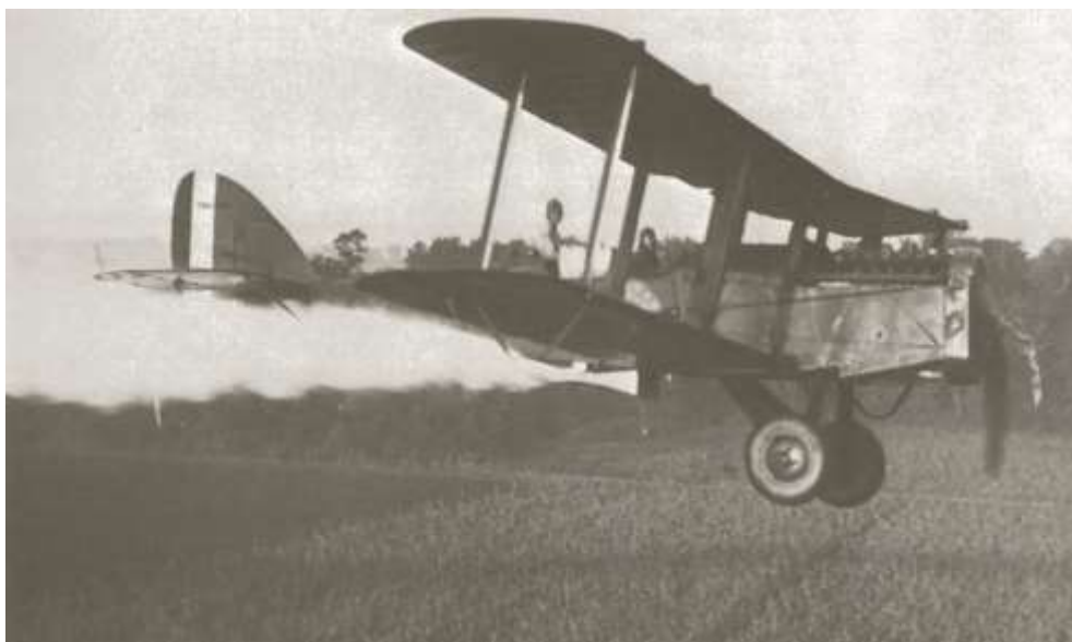
A modified Curtiss JN-6 "Jenny" airplane spreads lead arsenate dust over catalpa trees in Ohio in a successful experiment to kill sphinx moth larvae
