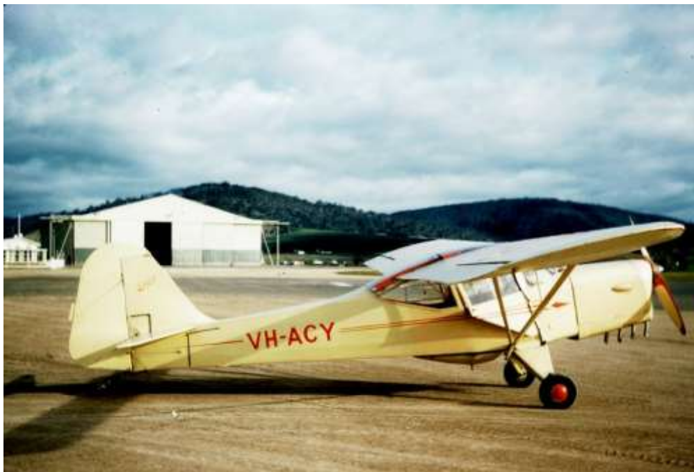
The Auster Aiglet VH-ACY used in the Swan Island rescue. The auxiliary fuel tank is visible under the fuselage
